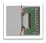
To open the ZiF-Connector you must pull the black bracket out.
